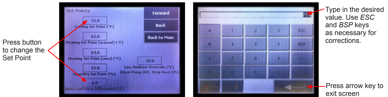
Figure 18. Set Point Selection & Adjustment Screens
