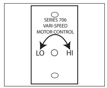
Figure 18. Indoor Blower Speed Control Adjustment Instructions
