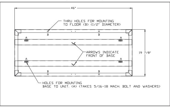
Figure 1a. Top View of Base Stand Part Number S/02093 (For 24/30/36/40)
