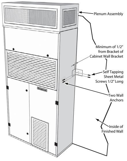
Figure 1. Installation of Wall Brackets (One on Each Side of Unit)
