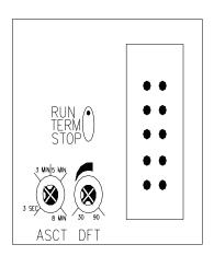
The micro switch has three positions – **RUN, TERM & STOP**. The switch should be in the **RUN** position during normal operation. **Term** is for operation from a remote terminal. **Stop** is no output/non-operational.
