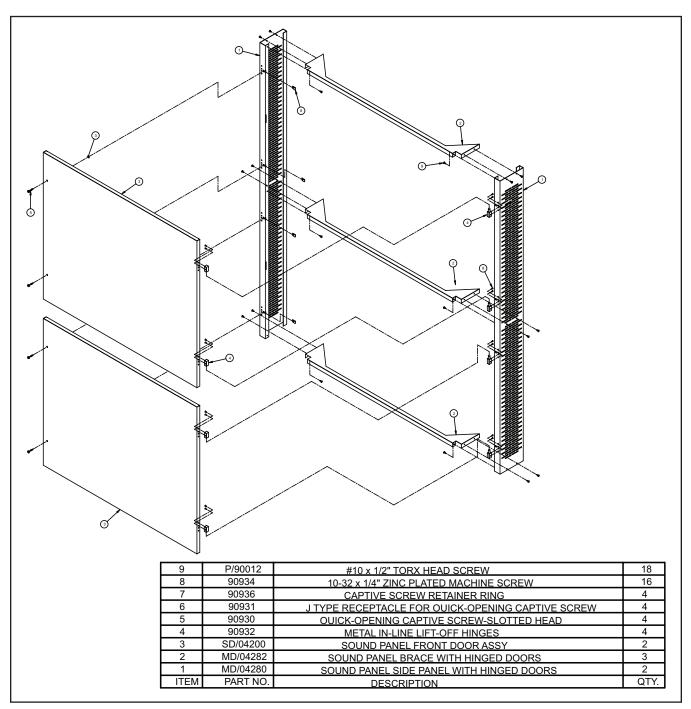
Figure 1. Sound Reduction Panel Installation
