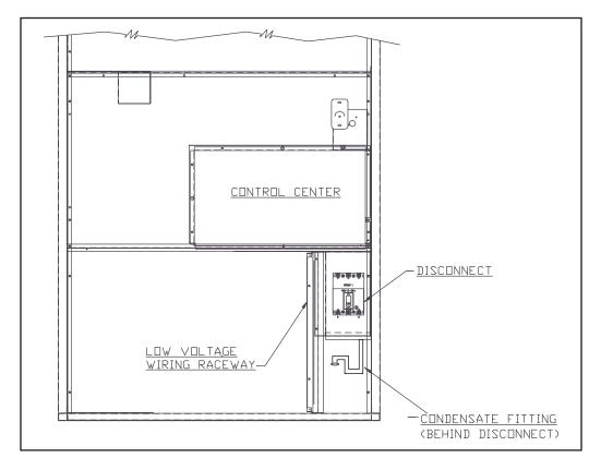
Figure 8b. Front View of Models 49/60 with Front Doors Open
