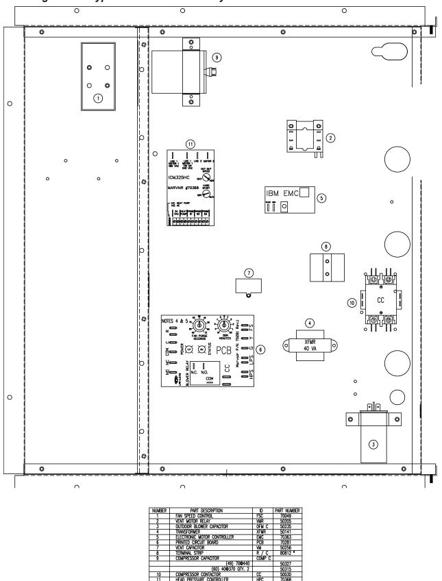
Figure 10. Typical Control Center Layout for Air Conditioner Models 49/60
