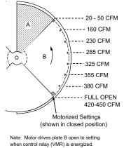
Motor drives plate B to the closed position when control relay (VMR) is deenergized.
