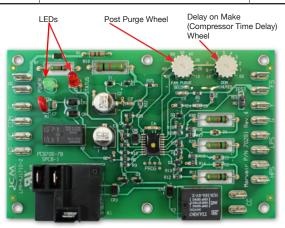
Figure 1. Electronic Control Board
