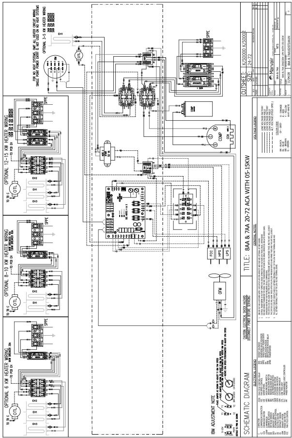
Figure 1a. Typical Electrical Schematic (Non-Economizer)
