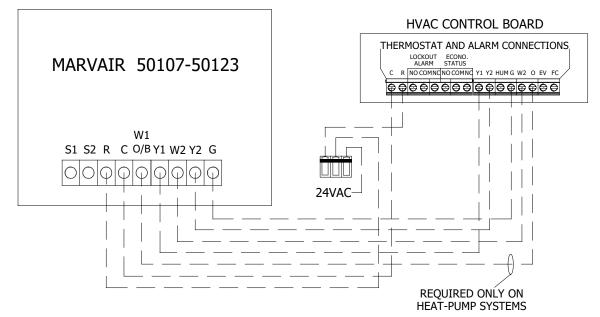
Figure 6b. Thermostat Connection Diagram
