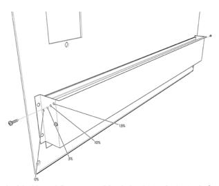
Figure 4. Fresh Air Hood Damper, Models 1024A-1060A & 2036A-2060A
