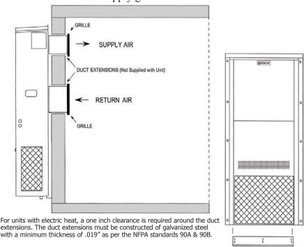
Figure 3. A/C Wall Mount Detail
