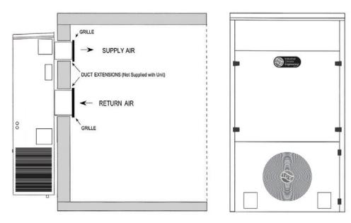
For units with electric heat, a one inch clearance is required around the duct extensions. The duct extensions must be constructed of galvanized steel with a minimum thickness of .019" as per the NFPA standards 90A & 90B.
