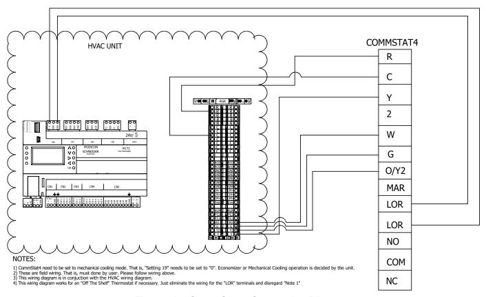
Figure 7b. CommStat 4 Connection Diagram
