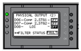
Note: In normal operation, the status of "DO8" is "OFF". If "DO8" is "ON" all outputs are turned off.
