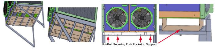
Figure 6a Unit Compression Support Examples
