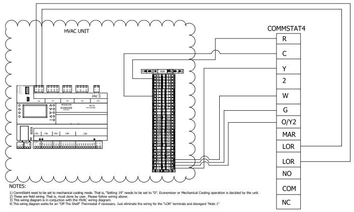
Figure 7b. CommStat 4 Connection Diagram
