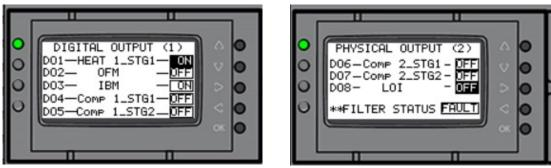
Note: In normal operation, the status of "DO8" is "OFF". If "DO8" is "ON" all outputs are turned off.
