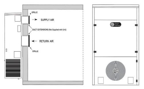
For units with electric heat, a one inch clearance is required around the duct extensions. The duct extensions must be constructed of galvanized steel with a minimum thickness of .019" as per the NFPA standards 90A & 90B.
