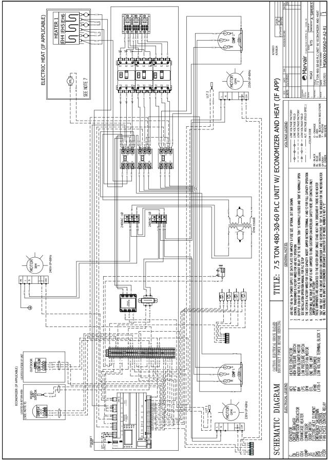
Figure 2a. Typical Electrical Schematic - MGH3090A
