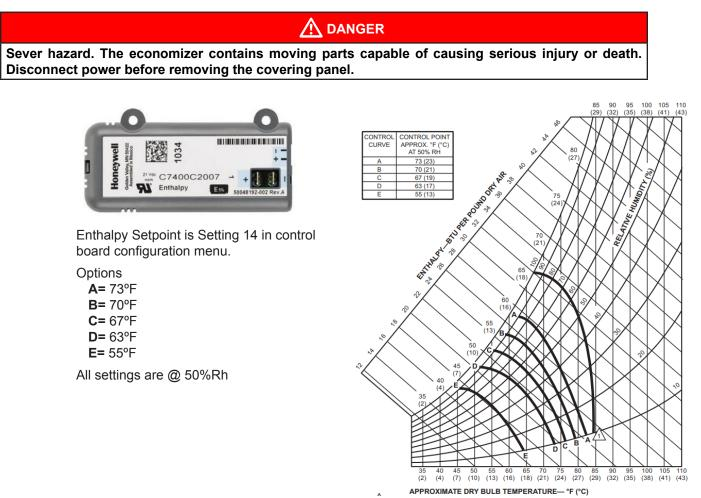
Figure 1. Enthalpy Sensor & Temperature Control Points
