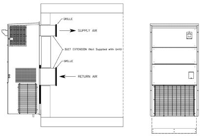
Figure 4. Mounting Unit on a Wall
