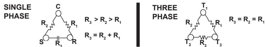
Resistance can be measured as shown above. Any deviation from above values could indicate a defective compressor.
