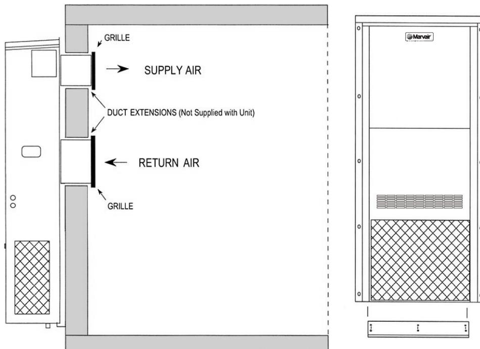
For units with electric heat, a one inch clearance is required around the duct extensions. The duct extensions must be constructed of galvanized steel with a minimum thickness of .019" as per the NFPA standards 90A & 90B.
