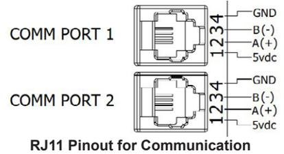
RJ11 Pinout for Communication
