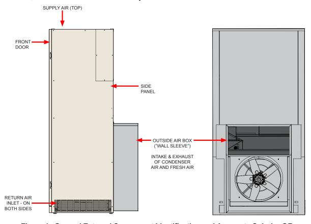
Figure 1. General External Component Identification and Access to Scholar QR
