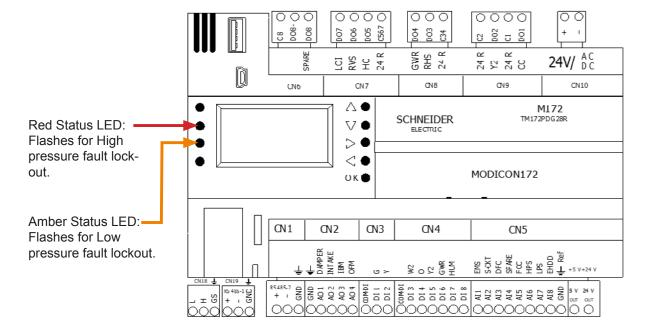
The following table describes the color and function for each of the PLC LEDs.
