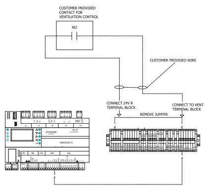
FOR CUSTOMER VENTILATION CONTROL, END USER WOULD NEED TO REMOVE FACTORY JUMPER WIRE #4 FROM "VENT" TO "24V R" TERMINAL BLOCK (DEPICTED ON THIS DIAGRAM) THEY WOULD ALSO PROVIDE THEIR ON NORMALLY OPEN CONTACT.
