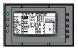
An output is a signal from the PLC to the Scholar QR heat pump or air conditioner or thermostat. All digital outputs on the PLC are 24V. These outputs are:
