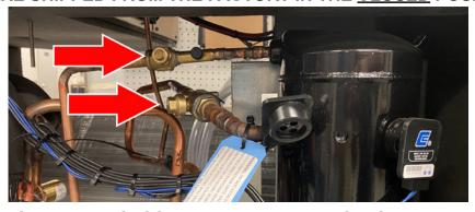
THE VALVES MUST REMAIN CLOSED UNTIL THE UNIT IS INSTALLED IN ITS PERMANENT UPRIGHT POSITION.
