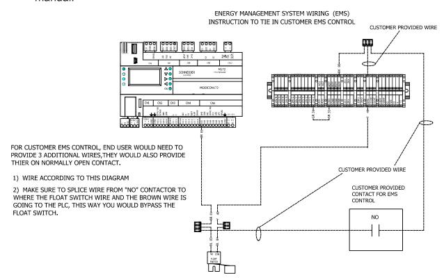
Figure 7. EMS Wiring Detail
