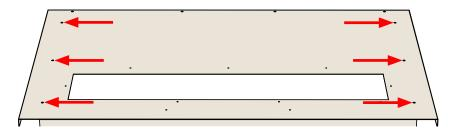
3. After the front panel has been removed, lift the plenum onto the top of the Scholar QR unit.
