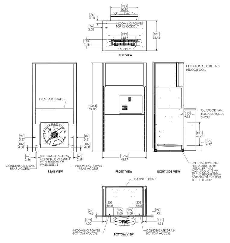
Figure 3. VDA2024/2036/2040 & VAA2030/2048/2060 w/Side Panels Removed
