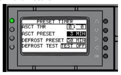
This screen involves the Anti-short Cycle, Defrost time and Defrost test setting.
