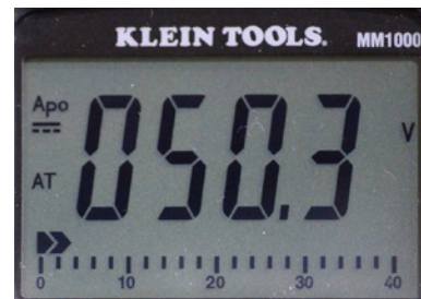
Indication of Positive DC Voltage
