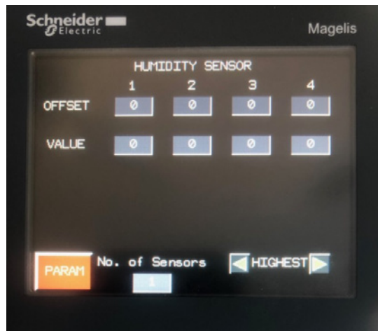
Figure 5 – “HUMIDITY SENSOR” Screen.
