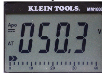
Indication of Positive DC Voltage
