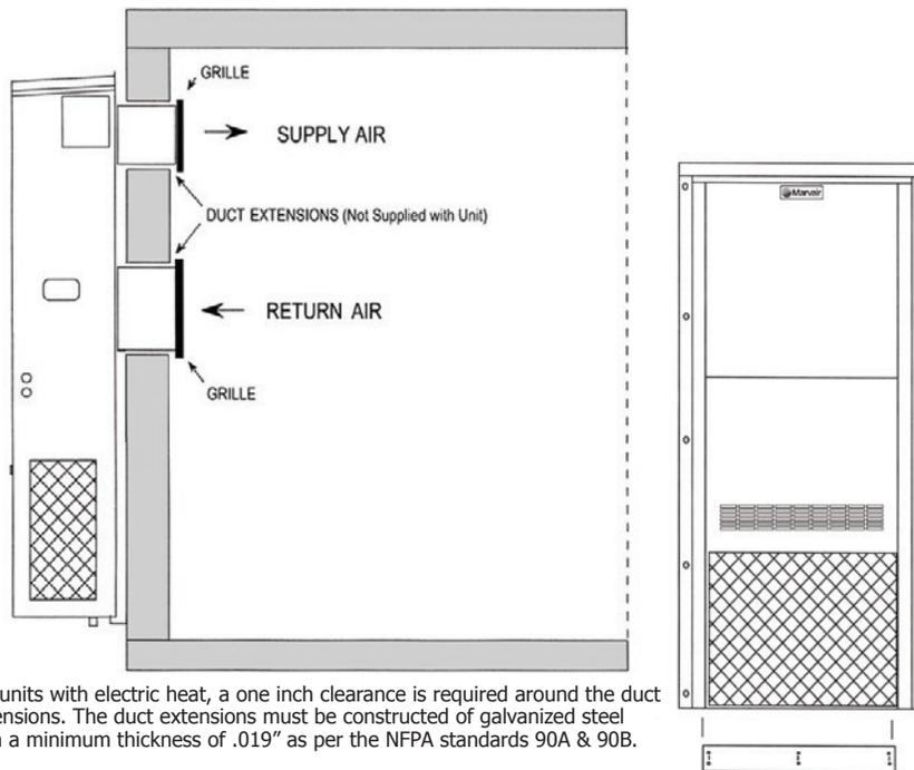
**Figure 3. A/C Wall Mount Detail**
