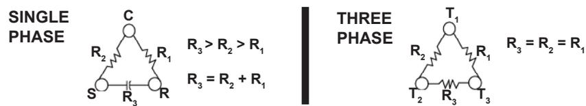
Resistance can be measured as shown above. Any deviation from above values could indicate a defective compressor.
