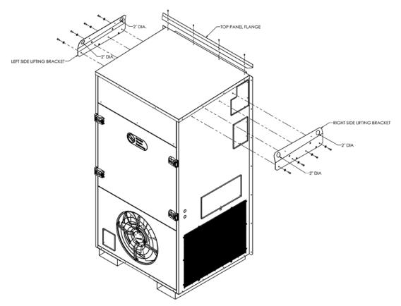
Figure 3 Top Flange and Lifting Bracket Installation (Typical)
