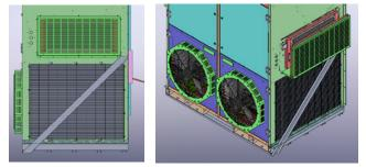
Figure 6b Unit Tension Support Examples
