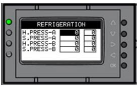
1. H. PRESS – A|B represents the liquid line temperature of circuit 1 and 2 respectively.
