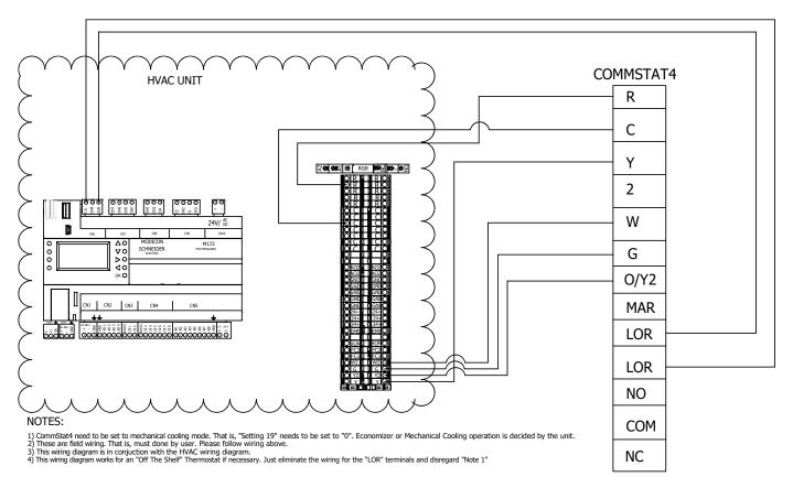
Figure 7b. CommStat 4 Connection Diagram
