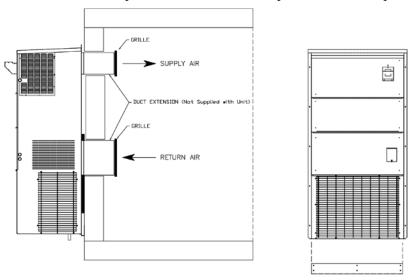
Figure 4. Mounting Unit on a Wall
