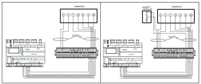
Figure 6a. Remote Wall Mounted Thermostat Wiring Detail
