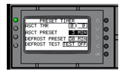
The Anti short cycle protects the system compressor from short cycling due to excessive on and off, this can happen when there is a fault or someone turning the system off and on for troubleshooting purpose etc. This timer starts timing when the compressor turns off and prohibits it from running again until the time period as elapsed.
