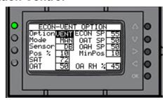
Scholar 2.0 are 2 stage units and Scholars with PLC and economizer option installed should use a 2 stage thermostat, to bring on Y2. If outside conditions are favorable the economizer will run to utilize "free" cooling. If the outside conditions are not favorable 1st stage mechanical cooling will operate. In the event the economizer cannot keep up to maintain the supply air temperature setting the unit will run 2nd stage mechanical cooling.
