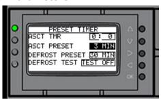
This screen involves the Anti-short Cycle, Defrost time and Defrost test setting.
