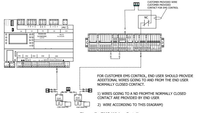
Figure 7. EMS Wiring Detail
