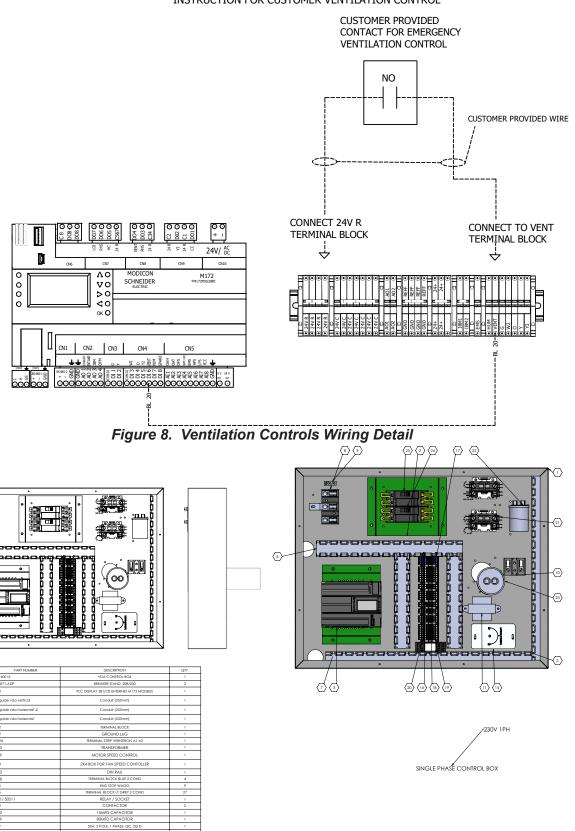
Figure 9a. Typical Control Center Layout for Single-Phase Scholar 2.0
