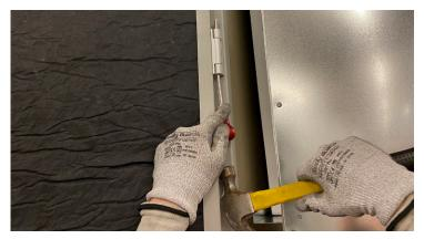
C. To remove the external side panel, first remove the 3 sheet metal secure screws located along the bottom edge of each side panel. Note: the securing screws should only be removed after the front doors are removed.
