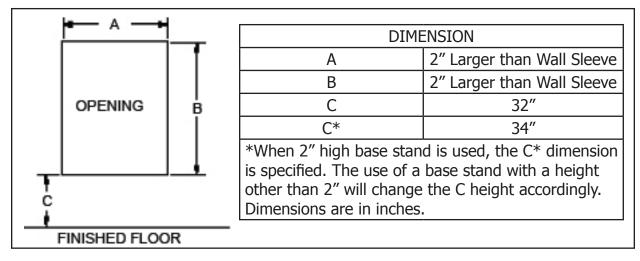
Figure 4. Wall Opening Dimensions for Scholar 2.0 Heat Pump and Air Conditioner
