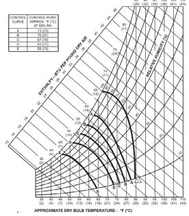
Figure 12. Enthalpy Sensor & Temperature Control Points
