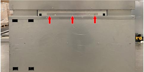
H. Using a mechanical lifting device, separate upper and lower sections.
