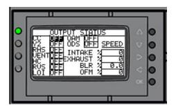
An output is a signal from the PLC to the Scholar 2.0 heat pump or air conditioner or thermostat. All digital outputs on the PLC are 24V. These outputs are:
